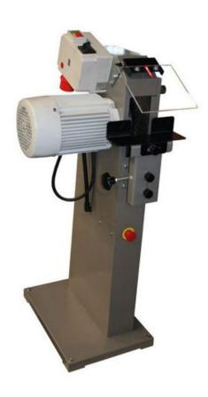
The Bauer BEF1 Deburring Machine 415V is ideal for the deburring of round/square tube and solid materials. A powerful motor drives a wire brush wheel and rapidly removes internal and external burrs in a single operation. The machine is produced with a two speed motor for effective finishing of ferrous and non ferrous metals.
