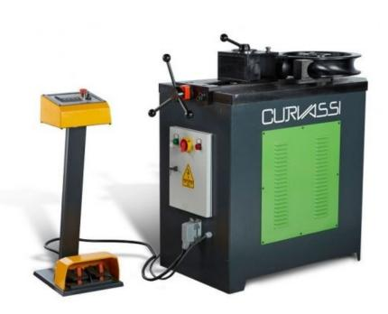
The Curvassi range of rotary tube bending machines have been designed for high quality bending of both metric and imperial tube sizes with a wall thickness sufficient to bend without a mandrel. Tooling can be supplied any tube diameter within the capacity of the machine and in a variety of centre line radii. Three models are available with tube bending capacities of up to 50mm, 60mm, 76mm and 114mm diameter, based on mild steel tube.
