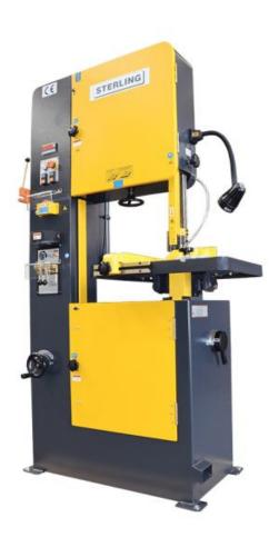
Sterling offer a wide range of sawing solutions including circular saws, horizontal bandsaws, twin column bandsaws and the SVR range of vertical bandsaws. The SVR range consists of four models of varying throat capacities. They are all equipped with blade shear, blade welder and grinder as standard equipment.
