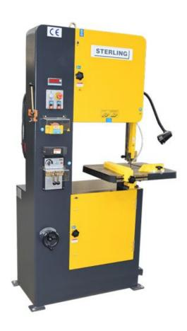
Sterling offer a wide range of sawing solutions including circular saws, horizontal bandsaws, twin column bandsaws and the SVR range of vertical bandsaws. The SVR range consists of four models of varying throat capacities. They are all equipped with blade shear, blade welder and grinder as standard equipment.
