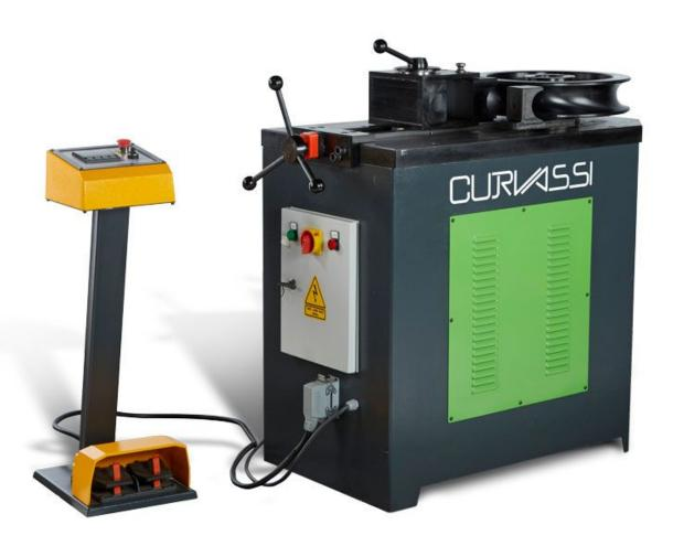
The Curvassi range of rotary tube bending machines have been designed for high quality bending of both metric and imperial tube sizes with a wall thickness sufficient to bend without a mandrel. Tooling can be supplied any tube diameter within the capacity of the machine and in a variety of centre line radii. Three models are available with tube bending capacities of up to 60mm, 76mm and 114mm diameter, based on mild steel tube.
