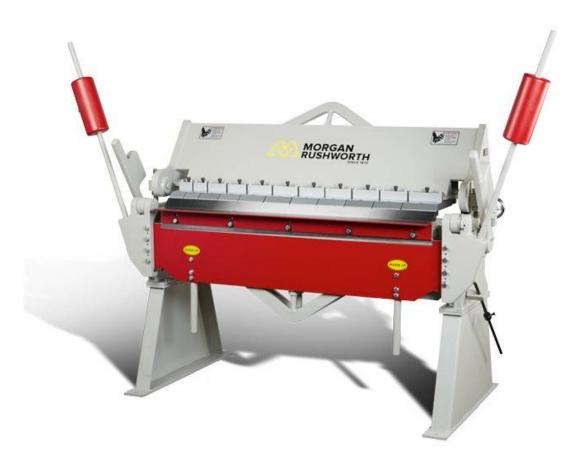
The heavy duty Morgan Rushworth Manual Box and Pan Folders are available in a range of sizes from 1270mm wide up to 3050mm. Intended for working with sheet metal material they have a capacity of up to 2.5mm thick except on the 3 metre model which accepts 2mm. All models feature 45° hardened and ground segmented fingers allowing both straight and box & pan folding in a range of materials. The counterbalance weights assist the operator, especially with repetitive cycles.
