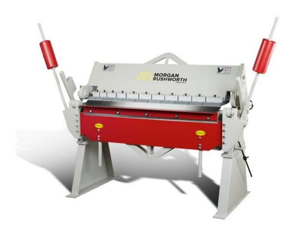
The heavy duty Morgan Rushworth Manual Box and Pan Folders are available in a range of sizes from 1270mm wide up to 3050mm. Intended for working with sheet metal material they have a capacity of up to 2.5mm thick except on the 3 metre model which accepts 2mm. All models feature 45° hardened and ground segmented fingers allowing both straight and box & pan folding in a range of materials. The counterbalance weights assist the operator, especially with repetitive cycles.
