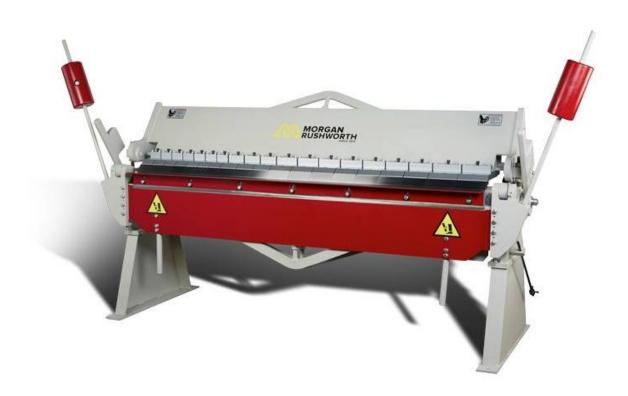
The heavy duty Morgan Rushworth Manual Box and Pan Folders are available in a range of sizes from 1270mm wide up to 3050mm. Intended for working with sheet metal material they have a capacity of up to 2.5mm thick except on the 3 metre model which accepts 2mm. All models feature 45° hardened and ground segmented fingers allowing both straight and box & pan folding in a range of materials. The counterbalance weights assist the operator, especially with repetitive cycles.
