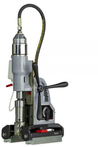
The portable Euroboor TUBE.55/AIR pneumatic drilling machine is equipped with an air-powered, spark-free motor and a non-electric, permanent dual magnet base. Connected to a compressor, it can be used for drilling on round as well as flat workpieces where electrical machines are less convenient or not allowed, especially in areas and spaces with potentially explosive atmospheres, such as offshore and petrochemical industries, as well as opencast mining.
