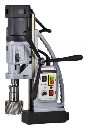
The Euroboor ECO.100/4 magnetic core drilling machine cuts holes up to  $\emptyset$  4" (100 mm) and is particularly suitable for tapping. This magnetic core drilling machine has an extremely powerful 17.3 A (1900 W) motor with a four-speed gearbox. The ECO.100/4 drilling machine benefits from a clockwise and counterclockwise rotating functionality and electronic speed adjustment
