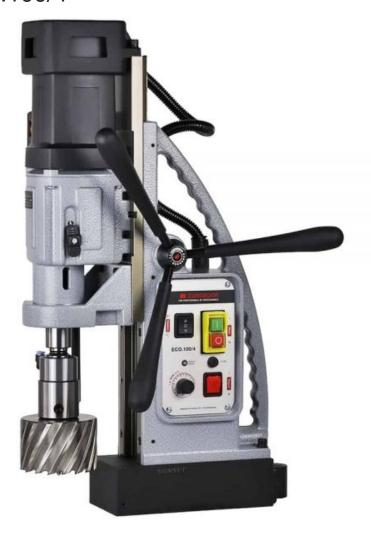
The Euroboor ECO.100/4 magnetic core drilling machine cuts holes up to Ø 4" (100 mm) and is particularly suitable for tapping. This magnetic core drilling machine has an extremely powerful 17.3 A (1900 W) motor with a four-speed gearbox. The ECO.100/4 drilling machine benefits from a clockwise and counterclockwise rotating functionality and electronic speed adjustment
