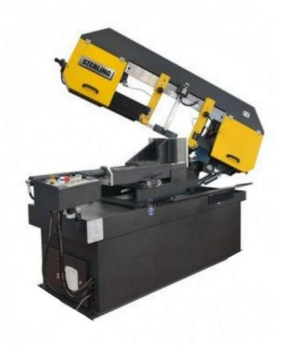
Sterling - SRA 320 DGSA horizontal band sawing machine, is ideal for angle cutting of materials with a varying number of cuts. It is possible to cut at variable angles between +45° and -60° by giving angle to the upper body of the machine. That machine makes the cutting hydraulically and automatically going up to the height after the cutting. The material is fed manually to the length stop and the cut is repeated.
