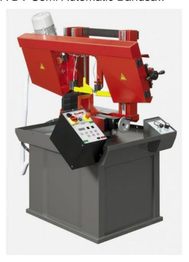
Semiautomatic band saw machine equipped with bow and vice movement at hydraulic control, automatic fast up/down bow movement controlled by feeler pin and cutting progress with infinitesimal adjustment. Twincolumn vertical descent. The machine has double safety button for cycle start and low voltage electrical system according to EC rules. The machine's design combined with the technical features grant high precision and absolute reliability.
