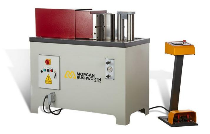
The Morgan Rushworth hydraulic horizontal bending machines are ideal for precision bending, straightening, punching and shearing. Available with capacities from 10 tonnes up to 100 tonnes and with a large range of optional tooling, these machines are capable of performing a whole variety of bending operations. The bending stroke and ram return positions are set using a simple digital programmer. Standard tools for bending flat bars are included.
