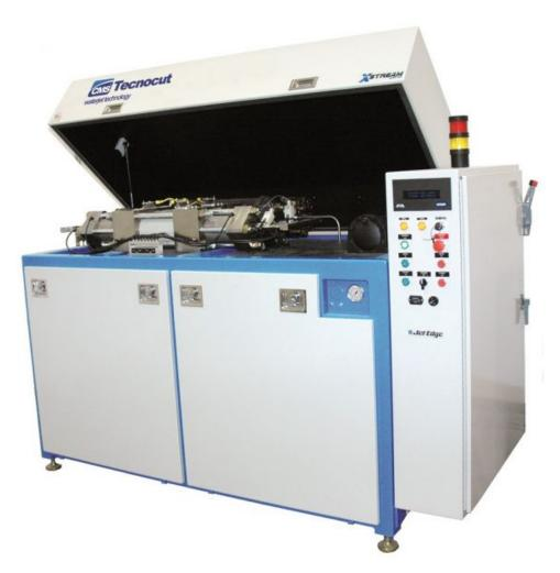
The X-Stream water jet pump produces 50% more pressure than a 60,000psi water jet intensifier pump, resulting in a 40-50% increase in productivity for many materials. The X-Stream supports a 75,000psi continuous operating pressure. Compared to a 60,000psi water jet pump, typical operating pressures of 75,000psi use 30% less water, 30% less power, and up to 50% less abrasive, resulting in a 40% reduction in operating costs. They typically reduce taper by up to 0.001".
