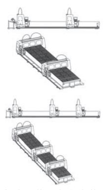
An advanced innovation that the Idea offers is its unique automated Dredge system. This utilises a heavy duty conveyor that runs in a valley in the centre of the tank and passes the used abrasive up and out of the tank into a waste container. The result is no manual abrasive removal which is often a labour intensive and dirty task that every waterjet operator generally has to undertake. This is a huge innovation and sets the Idea apart from other waterjet machines on the market.
