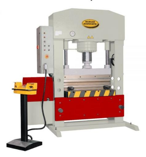
The heavily constructed PBH press brake model is of an H frame design and is fitted with heavy duty top and bottom press brake tools, ideal for a whole variety of heavier bending operations. These models feature adjustable limit switches for ram stroke and return, as well as twin guidance pistons in addition to the main ram. The machine operates at a safe working speed and is also fitted with a two handed control to ensure the operator is well away from the working area.
