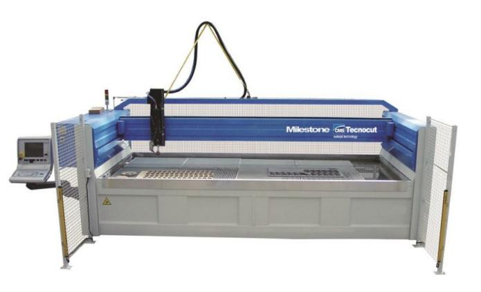
The CMS Milestone Waterjet cutting model represents the mid range offering from CMS providing additional process functionality with multiple cutting heads and 5 axis Bevel cutting capability.
