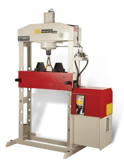
The HFP 1040/60 H frame press is ideal for a whole variety of bending, forming, pressing, straightening and a whole variety of operations. The hydraulic system is equipped with a manometer and a joystick lever to control the operation. A pair of V blocks are supplied as standard equipment.
