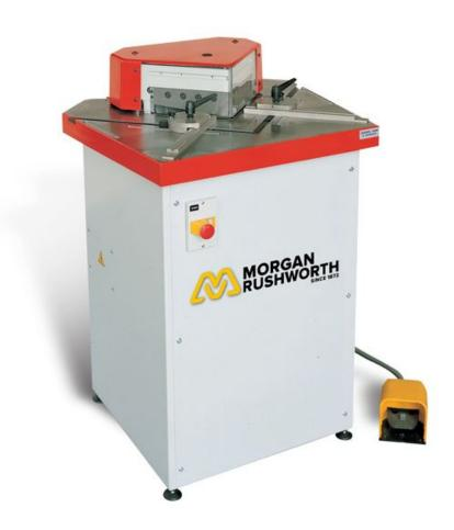
The HFA 220/8 hydraulic corner notching machine has a cutting capacity of 220mm x 8mm at a fixed angle of 90 Degrees. With a rigid head and GS500 cast iron workbench, these corner notchers are designed for a long working life.
