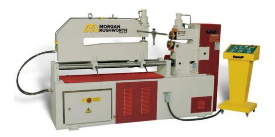
The Morgan Rushworth PCC 1200/3.5 Circle Cutting Machine is a powered model with a rigid construction. The machine is equipped with a reduction motor with brake and manual top cutter adjustment. The standard machine configuration allows the cutting of both standard circles and internal diameters to produce flanges.
