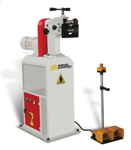
The Morgan Rushworth range of MS, PS and HPS swaging machines are available in manual, powered and hydraulic versions. Swaging machines are designed to form various shapes to sheet material and are particularly suited for tubular ductwork applications. Easily interchangeable rolls are included as standard equipment to form the specific shape required.
