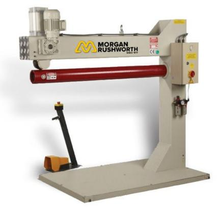
The Morgan Rushworth PSC pneumatic seam closer is designed to close a double seam join, with a professional uniform finish. The motorised top roll is pneumatically lowered onto the material and raised at the completion of the closed seam.
