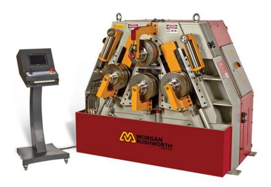
The Morgan Rushworth HSR-4 is a revolution in section bending. This unique new 4 roll machine brings all the benefits of 4 roll plate bending to section bending. The finished product has significantly reduced flat end, compared to 3 roll machines, due to the double pinching process. The optional touch screen NC Control allows for greater repeatability and accuracy with the ability to save down configurations.
