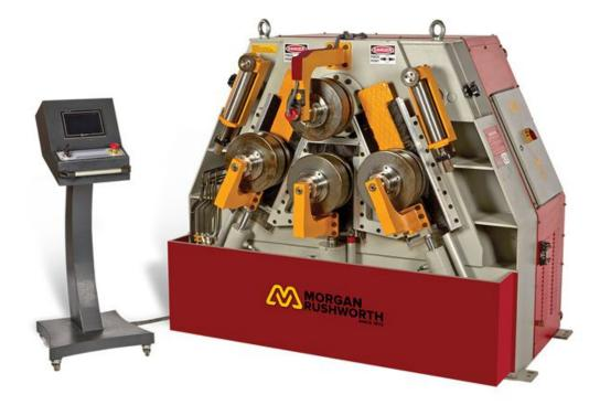
The Morgan Rushworth HSR-4 is a revolution in section bending. This unique new 4 roll machine brings all the benefits of 4 roll plate bending to section bending. The finished product has significantly reduced flat end, compared to 3 roll machines, due to the double pinching process. The optional touch screen NC Control allows for greater repeatability and accuracy with the ability to save down configurations.
