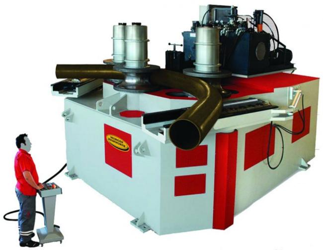
The Morgan Rushworth HSRD are one of the highest capacity ranges of section bending machines available. The largest HSRD 550/800 model can effortlessly roll 558mm x 22mm pipe and weighs a remarkable 61 tonnes. In all there are 6 models in the range starting with the 150mm model, all with powerful hydraulics controlling roll up and down translation, roll rotation and lateral guide roll movement.
