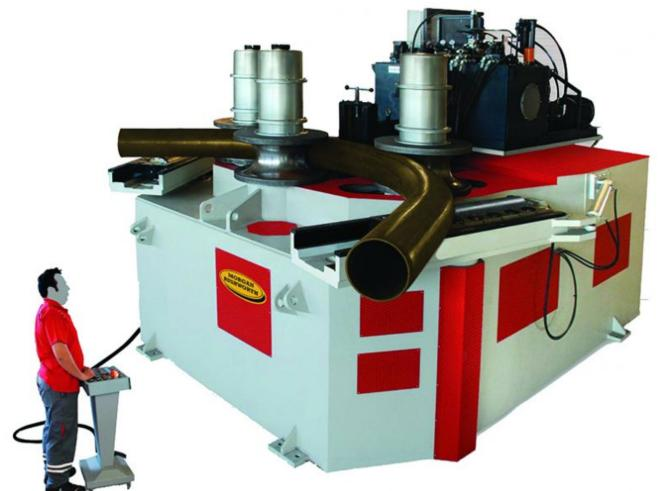
The Morgan Rushworth HSRD are one of the highest capacity ranges of section bending machines available. The largest HSRD 550/800 model can effortlessly roll 558mm x 22mm pipe and weighs a remarkable 61 tonnes. In all there are 6 models in the range starting with the 150mm model, all with powerful hydraulics controlling roll up and down translation, roll rotation and lateral guide roll movement.
