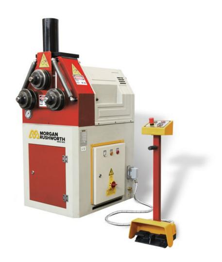
The Morgan Rushworth HSR 50/160 hydraulic section bending machine is designed to roll various material sections. This model has a single hydraulic ram to adjust the top roll, and can be operated in either vertical or horizontal plain. The standard rolls supplied with the machine are hardened and have been designed to bend most sections, avoiding the cost of additional tooling. Lateral guide rolls ensure straight and true bending, or if required can be adjusted in order to spiral the material.
