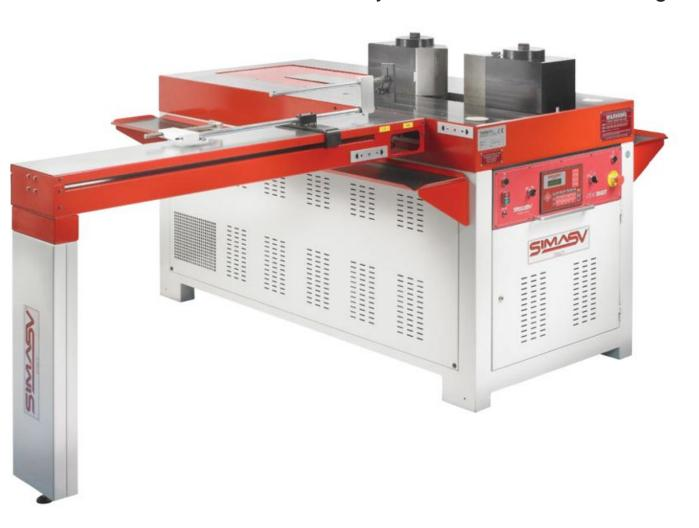
The T100 DIGIT 2 AXIS bending press allows the program and micrometer stroke adjustment through CN electronic positioner model SIMplylogik, even under the highest working pressure, so as to obtain the bending angle desired without practice tests and samples. Thanks to this system, the machine is ideal for either the production of prototypes or for the larger series.
