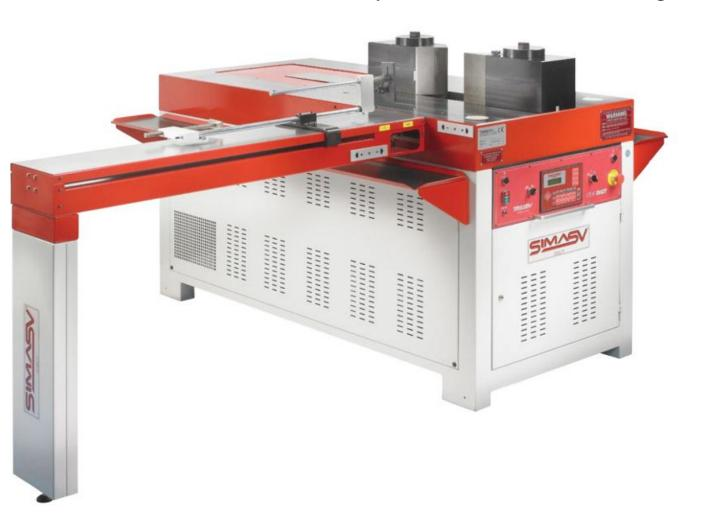
The T100 DIGIT 1 AXIS bending press allows the program and micrometer stroke adjustment through CN electronic positioner model SIMplylogik, even under the highest working pressure, so as to obtain the bending angle desired without practice tests and samples. Thanks to this system, the machine is ideal for either the production of prototypes or for the larger series.
