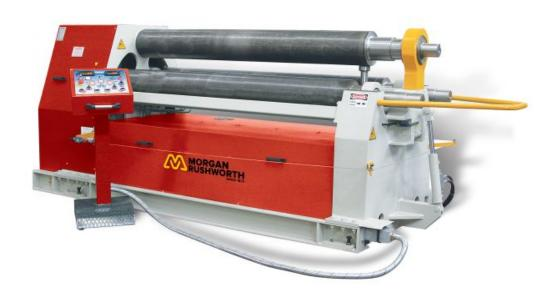
The Morgan Rushworth DPBH-3 hydraulic bending rolls are of the pyramid style with all three rolls hydraulically driven. The models with roll diameters up to 300mm are fitted with the type A shaft design with orbital action for up and down translation. The machines with roll diameters from 320mm to 550mm are equipped with type B shaft design with linear action for up and down translation. All models have hydraulic drop end and are supplied with DRO to indicate roll position.
