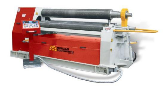
The Morgan Rushworth DPBH-3 hydraulic bending rolls are of the pyramid style with all three rolls hydraulically driven. The models with roll diameters up to 300mm are fitted with the type A shaft design with orbital action for up and down translation. The machines with roll diameters from 320mm to 550mm are equipped with type B shaft design with linear action for up and down translation. All models have hydraulic drop end and are supplied with DRO to indicate roll position.
