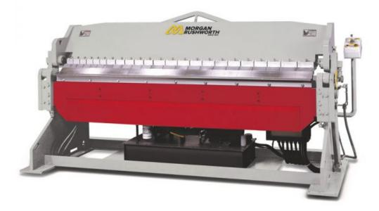
The Morgan Rushworth HBP range of hydraulic box and pan folders provide powerful folding with adjustable automatic angle setting device. The easy to use 4- way joystick controls beam clamping, folding, return and beam unclamping functions. This machine offers high speed, increased productivity and is a cost effective alternative to press brake machines. The HBP range have 45° angled fingers which are hardened and ground and supplied in varying widths for ultimate versitality.
