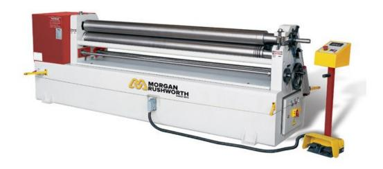
The Morgan Rushworth SBR Powered Top Roll to slip models range from 1mm - 5mm with a maximum bending length of up to 2050mm. The rugged heavy duty cast iron frame ensures long working life, while the asymmetric roll configuration enables pre bending capability.
