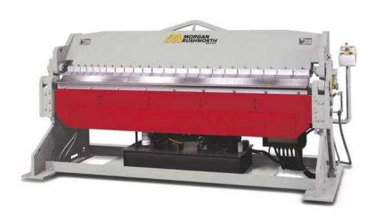
The Morgan Rushworth HBP range of hydraulic box and pan folders provide powerful folding with adjustable automatic angle setting device. The easy to use 4- way joystick controls beam clamping, folding, return and beam unclamping functions. This machine offers high speed, increased productivity and is a cost effective alternative to press brake machines. The HBP range have 45° angled fingers which are hardened and ground and supplied in varying widths for ultimate versitality.
