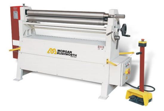
The Morgan Rushworth PBR Powered Top Roll to slip models range from 1mm - 5mm with a maximum bending length of up to 2050mm. The rugged heavy duty cast iron frame ensures long working life, while the asymmetric roll configuration enables pre bending capability.
