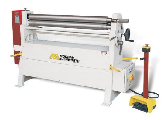
The Morgan Rushworth PBR Powered Top Roll to slip models range from 1mm - 5mm with a maximum bending length of up to 2050mm. The rugged heavy duty cast iron frame ensures long working life, while the asymmetric roll configuration enables pre bending capability.
