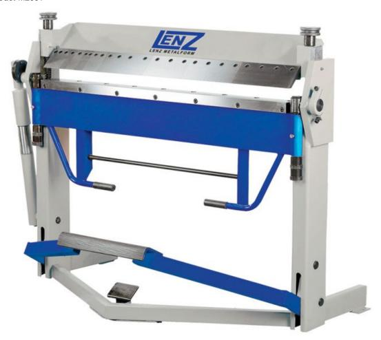
The Lenz Metalform LTBP 1270/20 box & pan folder is designed with removable fingers of varying widths for added versatility. The treadle system has been designed for hands free operation to position the material with the aid of a foot operated beam clamp. The two adjusting screws at the top of the machine can be altered according to material thickness. The fingers are machined to 45° providing a maximum bending angle of 135°.
