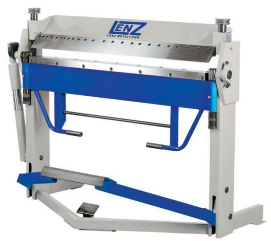
The Lenz Metalform LTBP 1020/2.5 box & pan folder is designed with removable fingers of varying widths for added versatility. The treadle system has been designed for hands free operation to position the material with the aid of a foot operated beam clamp. The two adjusting screws at the top of the machine can be altered according to material thickness. The fingers are machined to 45° providing a maximum bending angle of 135°.
