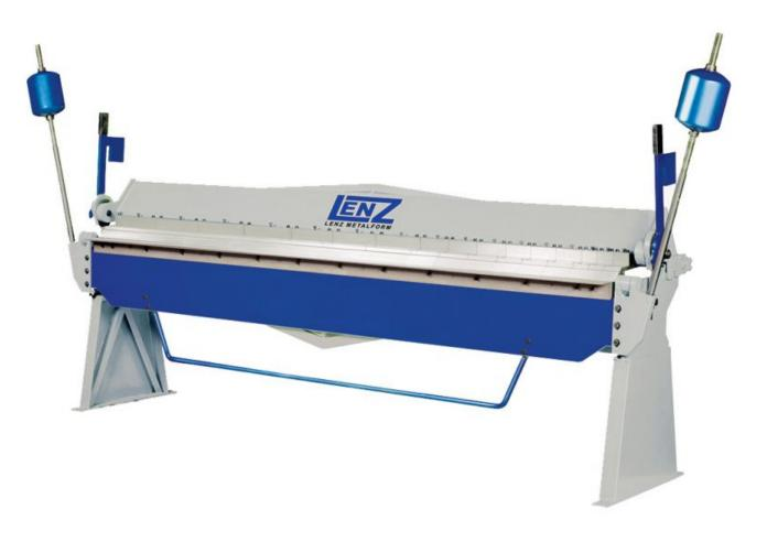
The Lenz Metalform LCBP 3050/2.0 Box and Pan folders has a 2mm bending capacity and a maximum bending length of 3050mm. The counter balance weights greatly assist the operator, especially during repetition cycles. The range has 45° angled fingers which are hardened and ground and supplied in varying widths for ultimate versitality.
