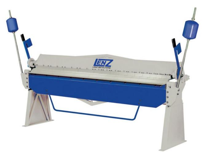
The Lenz Metalform LCBP 2540/2.5 Box and Pan folders has a 2.5mm bending capacity and a maximum bending length of 2540mm. The counter balance weights greatly assist the operator, especially during repetition cycles. The range has 45° angled fingers which are hardened and ground and supplied in varying widths for ultimate versitality.
