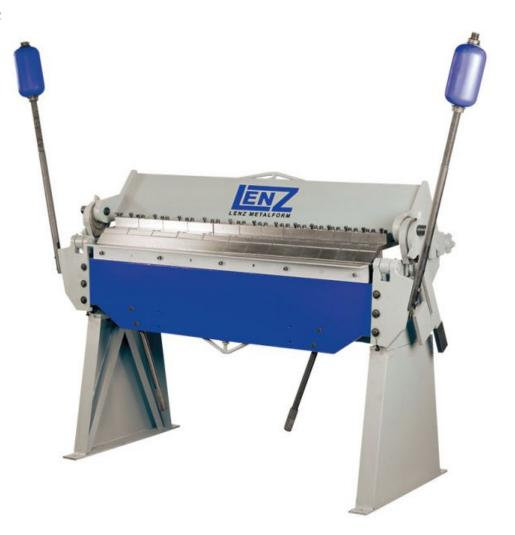
The Lenz Metalform LCBP 1270/2.5 Box and Pan folders has a 2.5mm bending capacity and a maximum bending length of 1270mm. The counter balance weights greatly assist the operator, especially during repetition cycles. The range has 45° angled fingers which are hardened and ground and supplied in varying widths for ultimate versitality.
