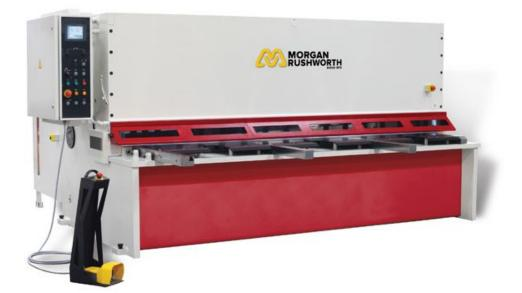
The powerful BHGS range of hydraulic swing beam guillotines are equipped with a high visibility front guard design consisting of a fixed guard with windows. All machines are fitted with stainless steel quality cutting blades as standard, giving flexibility to cut a range of materials without detriment to blade life.
