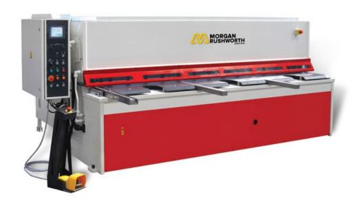
The HSGS range of hydraulic swing beam guillotines are equipped with a high visibility front guard design consisting of a fixed guard with windows. All machines are fitted with stainless steel quality cutting blades as standard, giving flexibility to cut a range of materials without detriment to blade life.
