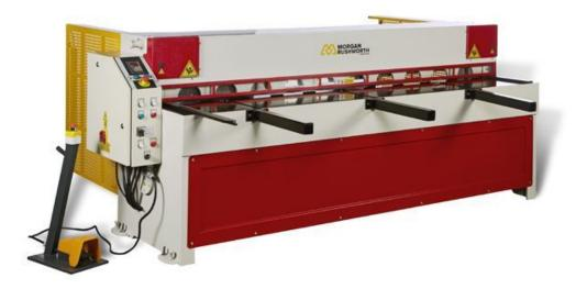
The RGMS range of powered mechanical guillotines are designed for fast accurate cutting of sheet material. They are available in a wide range of capacities with either the standard manually operated backgauge or the optional advanced Elgo NC programmable powered backgauge.
