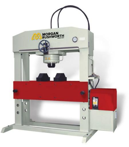
The HFPV H frame presses are ideal for a whole variety of bending, forming, pressing and straightening operations. These models include all the features of the popular HFP models with the addition of side to side ram movement across the width of the machine. The hydraulic system is equipped with a manometer and a joystick lever to control the operation. A pair of V blocks are supplied as standard equipment.
