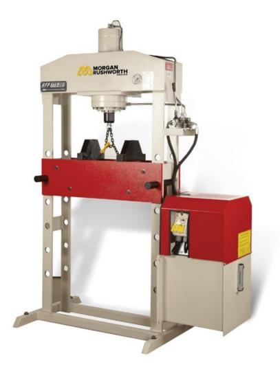
The HFP 1570/150 H frame press is ideal for a whole variety of bending, forming, pressing, straightening and a whole variety of operations. The hydraulic system is equipped with a manometer and a joystick lever to control the operation. A pair of V blocks are supplied as standard equipment.
