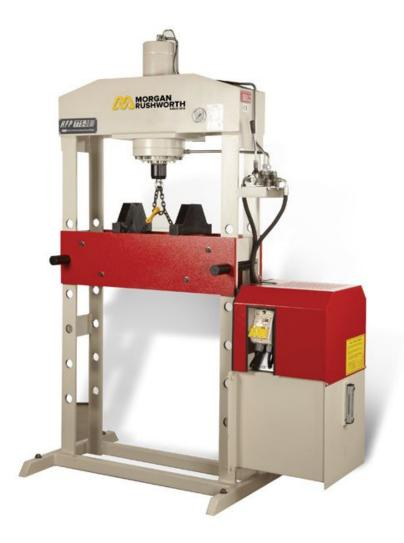
The HFP 775/30 H frame press is ideal for a whole variety of bending, forming, pressing, straightening and a whole variety of operations. The hydraulic system is equipped with a manometer and a joystick lever to control the operation. A pair of V blocks are supplied as standard equipment.
