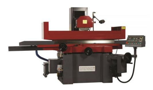
The Brenner HAD Rapid Feed Surface Grinding Machines are produced with highly rigid cast iron body ensuring maximum rigidity. These models feature automatic feed on longitudinal, cross and vertical axes. They are designed to operate with low vibration, high accuracy and low maintenance requirements and include centralised one-shot lubrication. A permanent magnetic chuck, coolant system and a halogen working light are all standard equipment.
