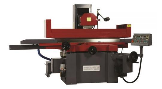
The Brenner RAD Rapid Feed Surface Grinding Machines are produced with highly rigid cast iron body ensuring maximum rigidity. Both the longitudinal and cross feeds are automatic while the vertical feed is manual with a rapid feed function. They are designed to operate with low vibration, high accuracy and low maintenance requirements and include centralised one-shot lubrication. A permanent magnetic chuck, coolant system and a halogen working light are all standard equipment.
